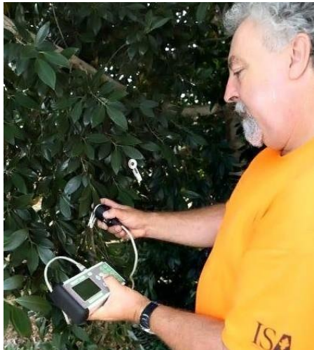
Figure 8 - Using the Handy PEA fluorimeter to measure chlorophyll fluorescence values.
